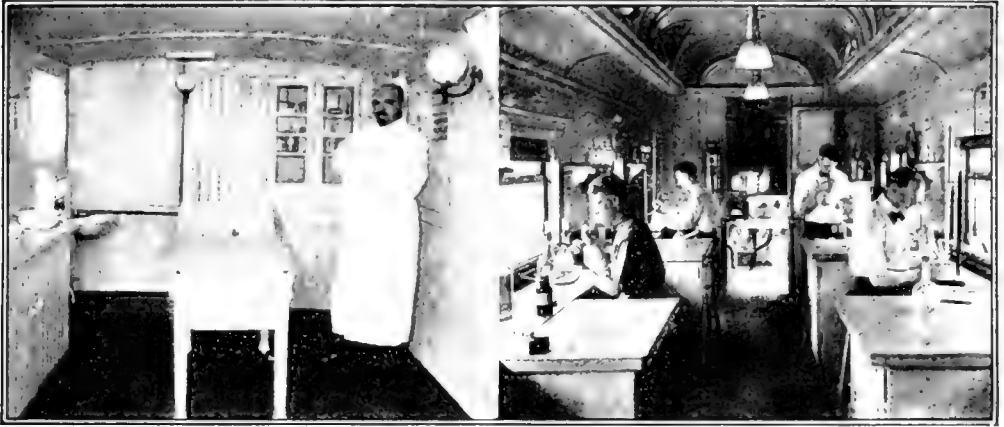
A traveling emergency hospital with an operating table, closets for medicines, washbasins, sleeping cots and all conveniences for giving first aid to the injured
